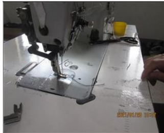
Photo of non-conformity NC Finger guard was installed ineffectively.JPG
